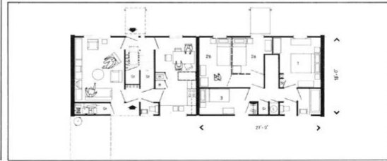
1 Five Person House, Midland Housing Consortium, 1967. 'This house has been designed to meet the needs of a fully segregated, dual access layout' – the nature of contemporary-house architecture is concealed within subtle tautologies like this.
